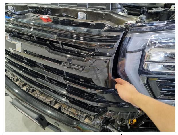
14. Pull outwards and release the clips securing the grille to the vehicle. Set aside in a safe place for later.
