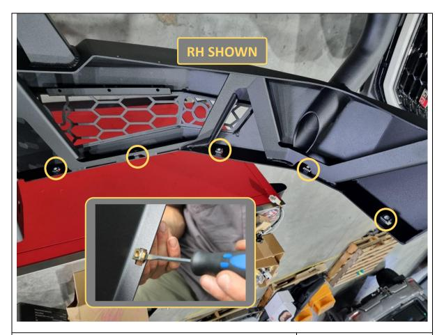
98. Fit 5x M6 cage nuts into the rectangular slots on the bottom of the bar wing.
