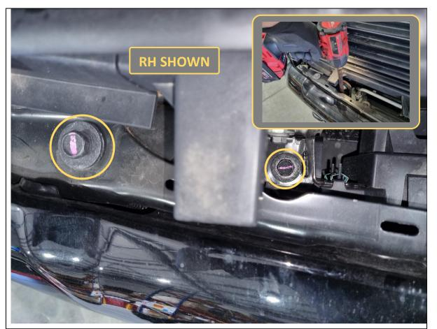
18. Looking down on the top lip of the bumper, remove 4x 18mm hex bolts securing the top bumper support brackets.
