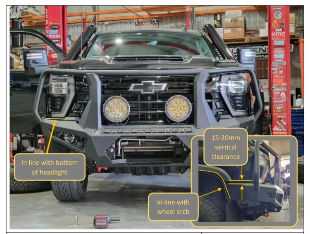
108. With assistance, from another person, align the bar with the edges of the vehicle. Adjust such that the clearances are neat, and the bar is symmetric left/right on the vehicle.
