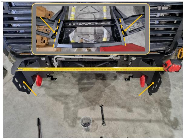
37. Measure the horizontal distance between the outside faces of uprights on bar using tape measure. Write distance below for reference if required.
